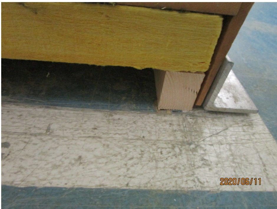
Figure 2 – Specimen and edge seal configuration, air space between specimen and test surface
