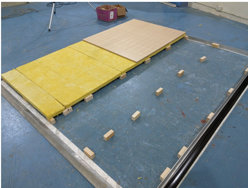
Figure 4 – Specimen panels and base layer fiberglass partially installed over spacers
