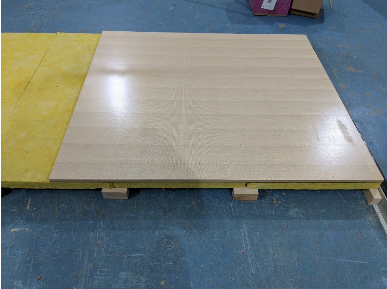
Figure 5 – Specimen panels and base layer fiberglass partially installed over spacers
